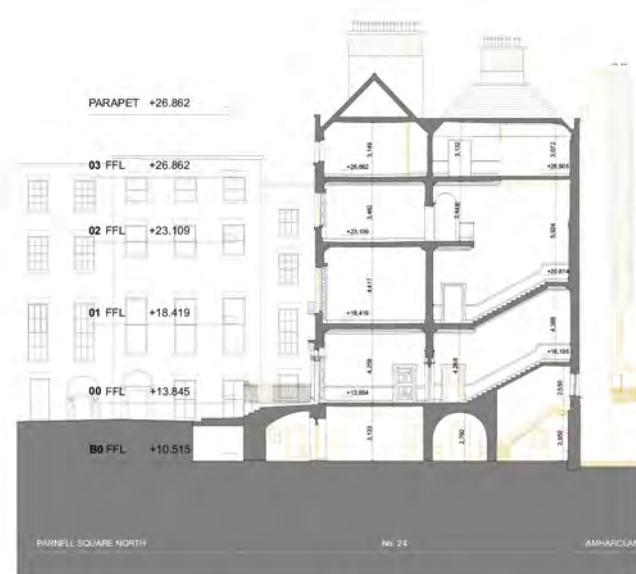
SOUTH-NORTH CROSS SECTION THROUGH NO 24
