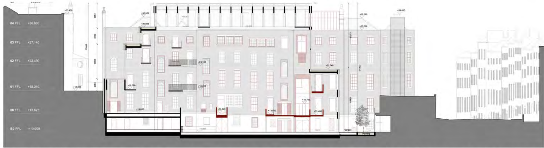
EAST-WEST SECTION THROUGH NEW BUILD SHOWING REAR (NORTH) FACADE OF EXISTING HOUSES AND CONNECTING BRIDGE LINKS
