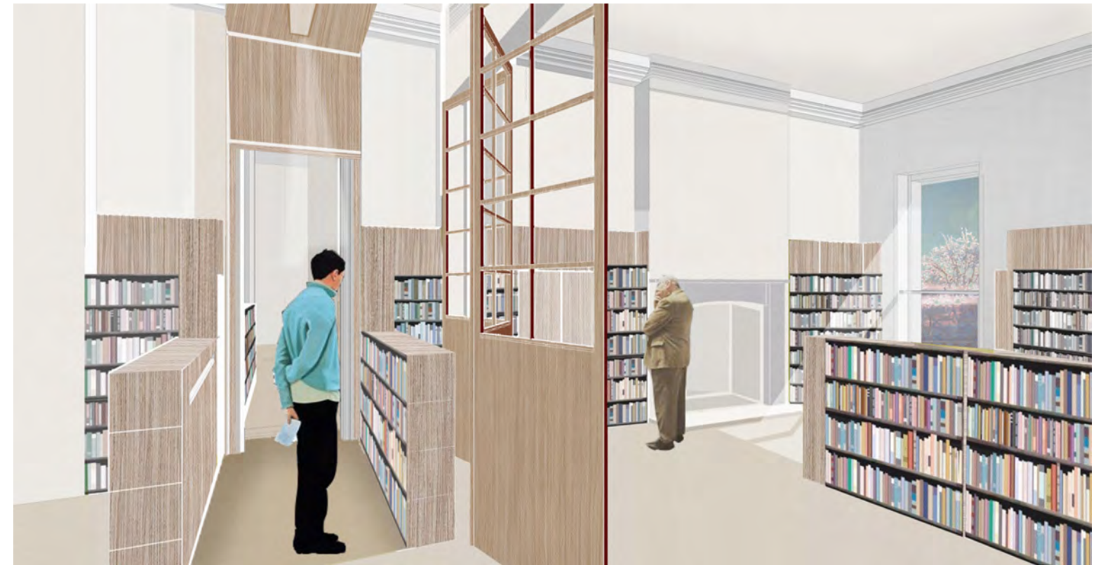
Fig 7.15: Concept sketch showing new ramps and opening in party walls; folding doors from Colaiste Mhuire retained
