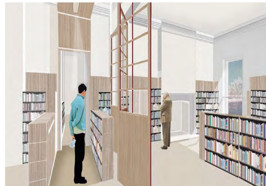
Figs 6.11: Insertions & Installations: Sketch image showing proposed new furniture/fitings (installations) and ramps (insertions) treated as new, reversible, elements within the historic rooms
