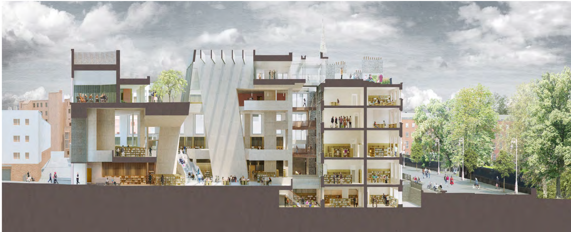
Fig 7.10: Sectional perspective through the proposed new library showing, from left, the large new rooflit library volume with its pocket gardens and public entrance from Bathesda Place; the more intimate, yet grand, Georgian proportioned rooms (section through No 25), which overlook Parnell Square with the proposed public terrace at roof level, availing of the already altered roovescape and, the public realm with widened pavements and enhanced pedestrian environment.
